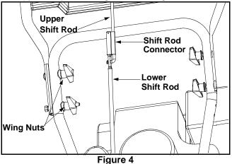
• Slide the shift rod connector down over the end of the lower shift rod. Tap the connector until it **locks** on the lower shift rod. See Figure 4.
